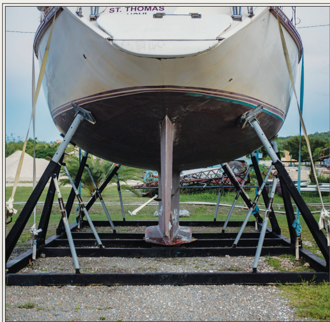
Two successful methods of securing boats ashore during hurricane season: Lloyd's-approved cradles are considered to be one of the strongest options (left). Hurricane pits reduce windage and the forces on stands and supports (right).
