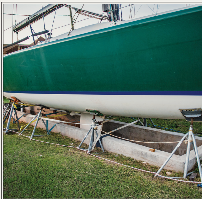
Two successful methods of securing boats ashore during hurricane season: Lloyd's-approved cradles are considered to be one of the strongest options (left). Hurricane pits reduce windage and the forces on stands and supports (right).
